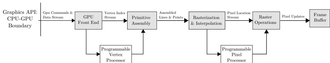
Figure 3.1: A conceptual image of the programmable graphics pipeline [12].
