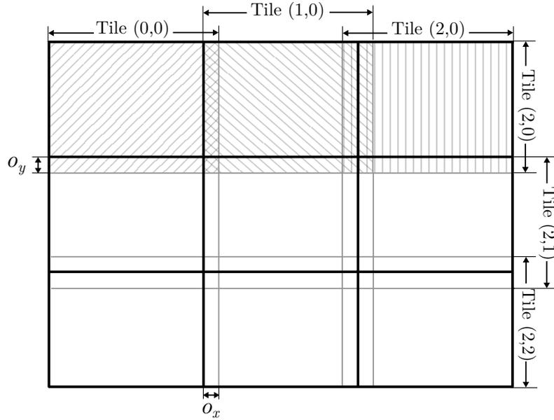
Figure 4.5: An example of dividing an image into three tiles horizontally and vertically.
