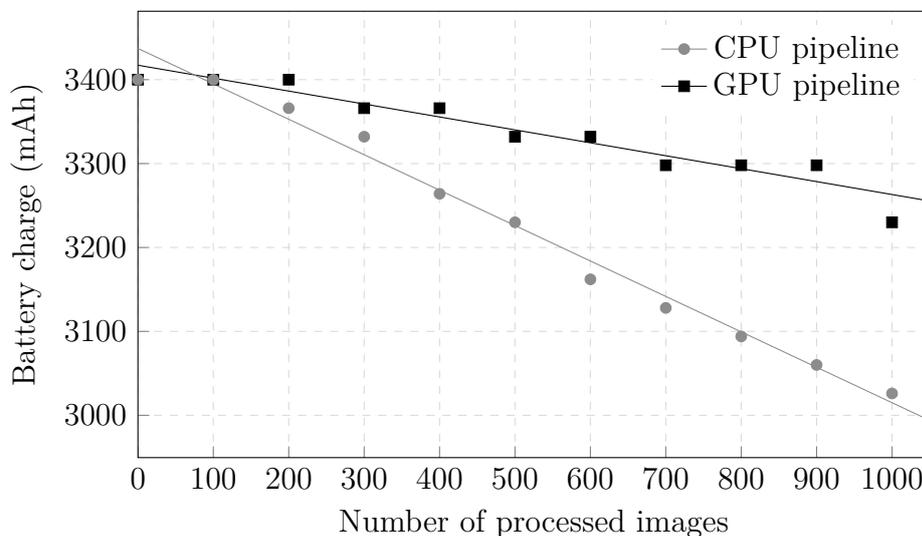
Figure 6.4: The battery charge of the test device when 1000 images were processed consecutively.
