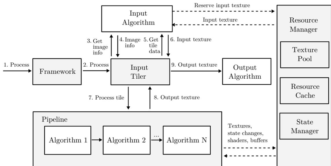
Figure 4.3: A high level structure and the processing flow of the framework.
