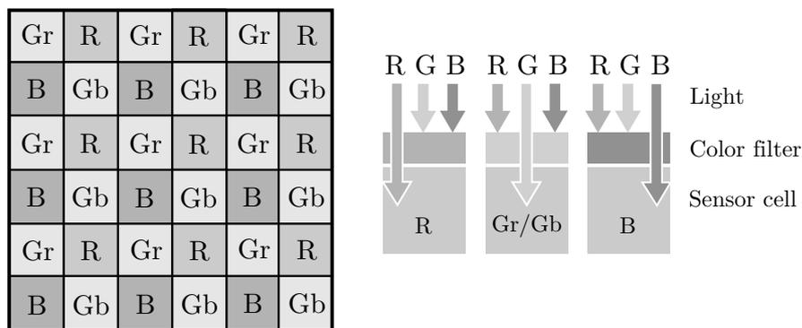
Figure 2.3: A Bayer pattern color filter array and the structure of different color pixels.
