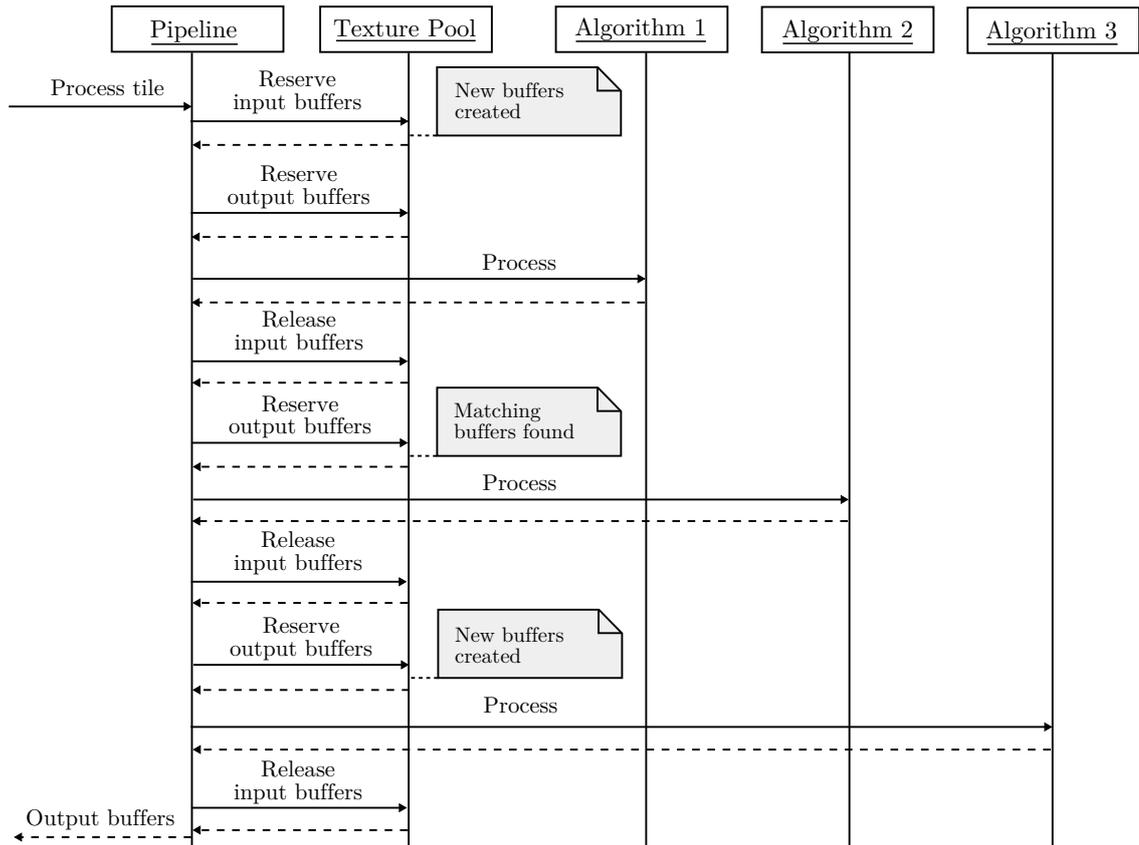
Figure 4.8: The processing flow inside the pipeline component.
