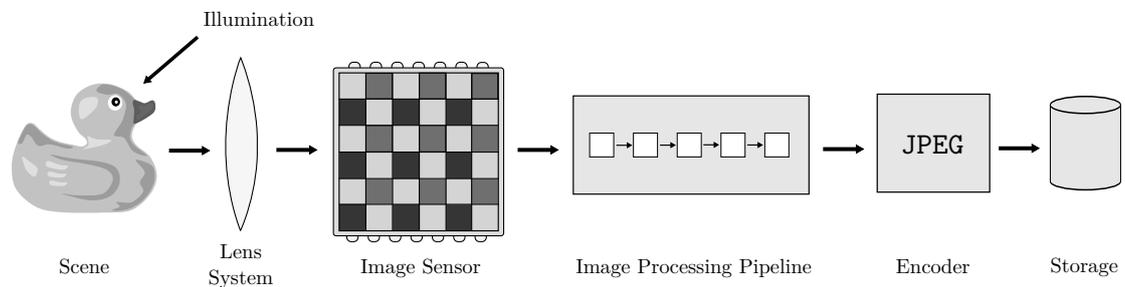
Figure 2.1: The components of a digital still camera.
