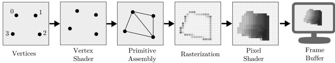
Figure 3.2: Vertices during different stages of the graphics pipeline.
