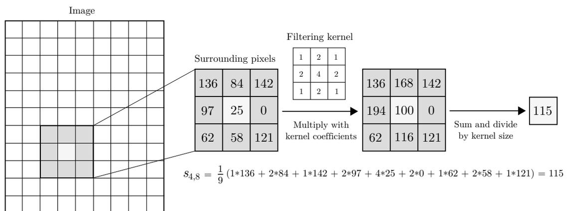
Figure 2.7: A simple blur effect using a 3x3 filtering kernel.
