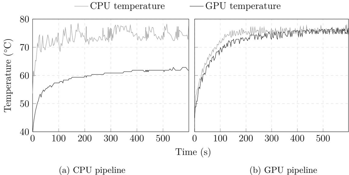
Figure 6.1: Measured GPU and CPU temperatures for (a) CPU implementation and (b) GPU implementation during processing.
