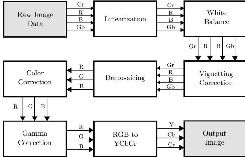
Figure 2.9: Algorithms in a typical image processing line [11].
