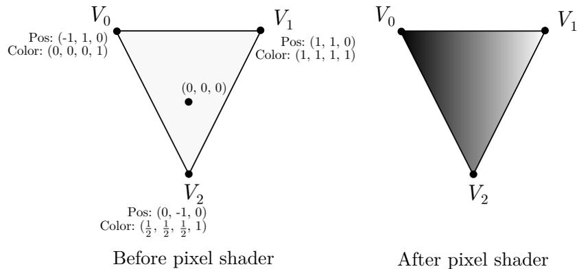
Figure 3.3: The output of a pixel shader that sets the color of the pixel directly to the color passed from the vertex shader.
