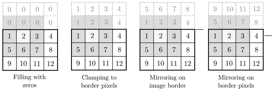
Figure 2.8: Different methods for processing border pixels when a processing kernel is used.
